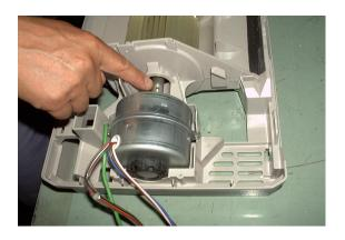
③ Pull out the fan boss from the fan motor shaft, and then pull out the fan to the left.
